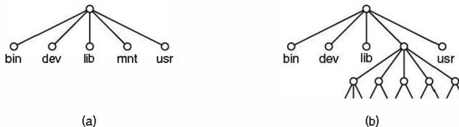
Figure 1-22. (a) File system before the mount. (b) File system after the mount.
