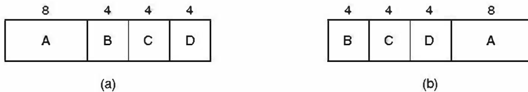
Figure 2-40. An example of shortest job first scheduling. (a) Running four jobs in the original order. (b) Running them in shortest job first order.
